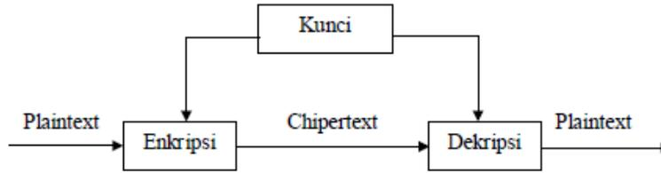
Figure 1. Symmetry algorithm
