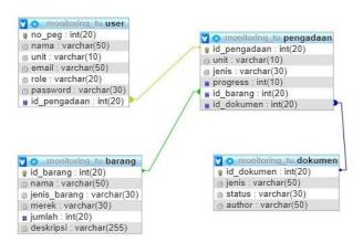
Figure 3. Design of ERD
