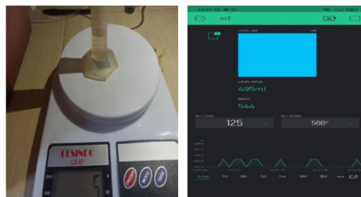
Figure 3. Infusion Bag Fluid Volume Reading
