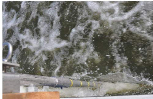
An oscillator of an echo sounder was attached to the other end of the pole beneath the water surface (b)
