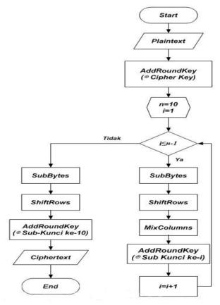
Figure 2. AES Algorithm Encryption Process Diagram
