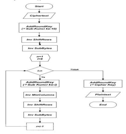
Figure 3. AES Algorithm Decryption Process Diagram
